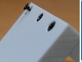
Uniboard is easy to work with and can be cut, routered, drilled, & mechanically fastened with standard hardware materials such as screws and regular construction adhesives.
